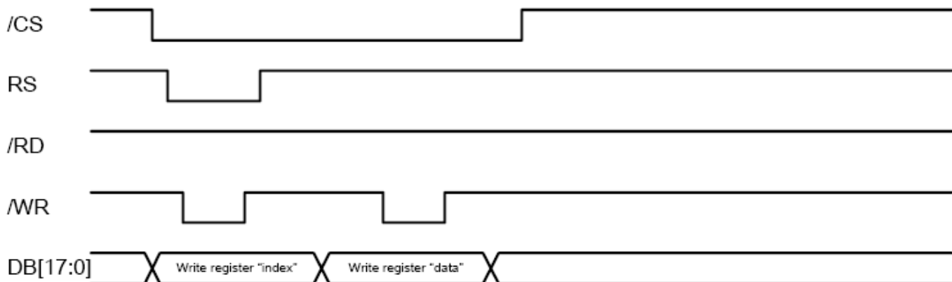
Figure 5.2 i80 18-bit System Bus Interface Timing
