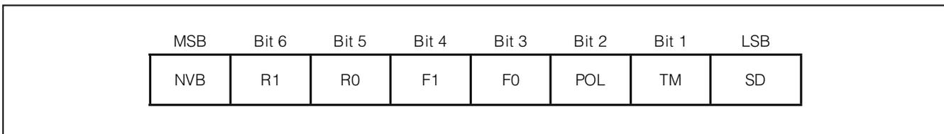
Figure 5. Configuration Register
