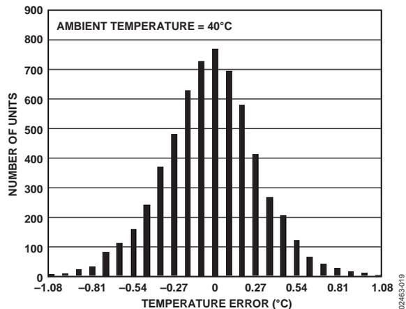
Figure 19. Ambient Temperature Error @ 3 V
