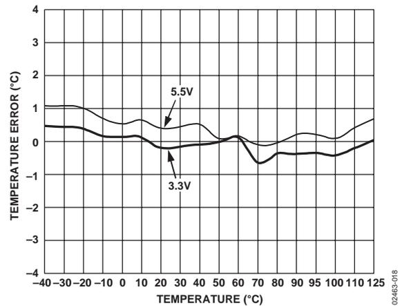
Figure 18. Typical Temperature Error @ 3.3 V and 5.5 V
