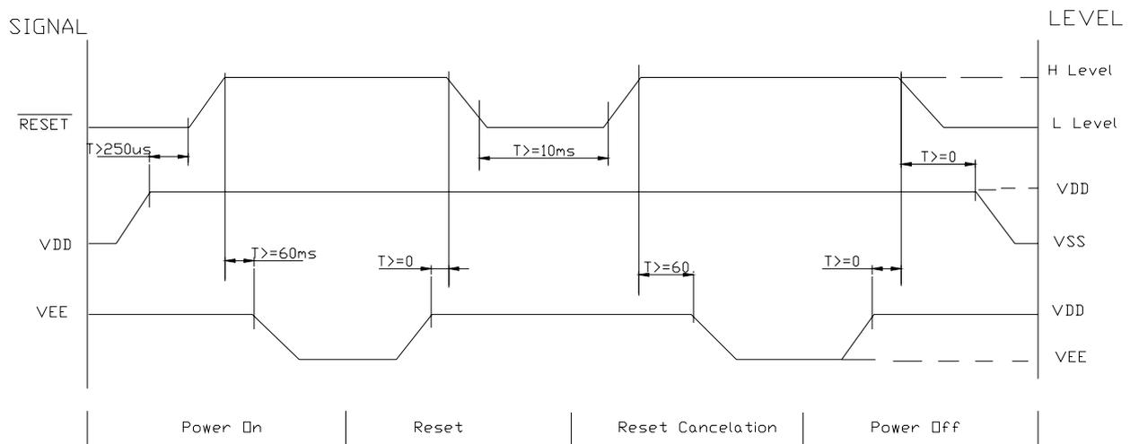
Please maintain the above sequence when turning on and off the power supply of the module.
