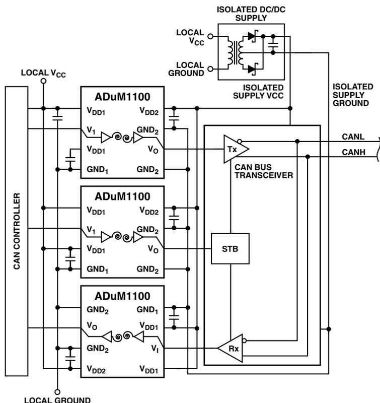
Figure 5. CAN Bus Isolation Using Three ADuM1100s
