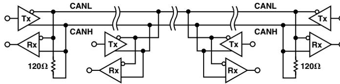
Figure 2. CAN Bus Network
