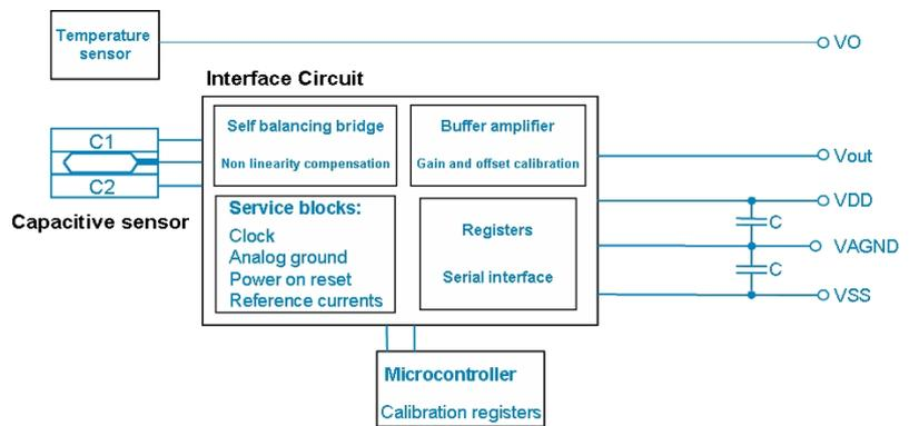
It is strongly recommended to use decoupling capacitors [C] of 1 $\mu$ F each between VDD and VAGND and between VAGND and VSS, placed as close as possible from the accelerometer. COG or X7R @ 5% capacitor types are recommended. On top, the VAGND track should be as short as possible. Any other setup will potentially affect the bias calibration and stability.
