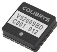
The VS9000 vibration sensor is a single axis MEMS capacitive accelerometer based on a bulk micro-machined silicon element specifically designed for large and flat frequency response, a low power ASIC for signal conditioning, a micro-controller for storage of compensation values and a temperature sensor. The product is low power, fully calibrated, robust and extremely stable and the electronic configuration provides a solid power on reset and ensures a full protection against brown-out...
