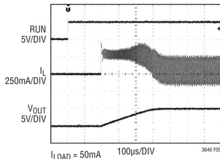
Figure 5. Start-Up Waveform
