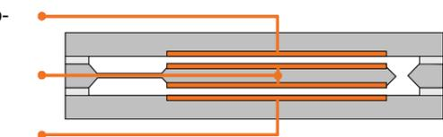
Fig. 2 : Cross section of a Colibrys accelerometer
