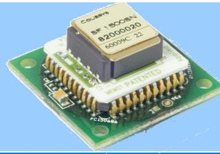
MEMS Capacitive Accelerometers
