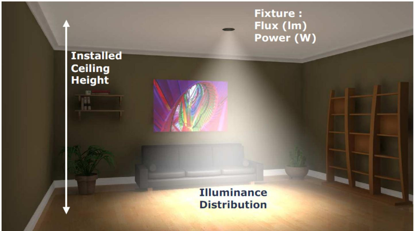
**Figure 1 - Critical Characteristics for Example CFL Downlight**
