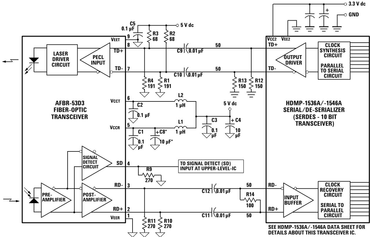
Figure 3. Recommended Gigabit/sec Ethernet AFBR-53D3 Fiber-Optic Transceiver and HDMP-1536A/1546A SERDES Integrated Circuit Transceiver Interface and Power Supply Filter Circuits.
