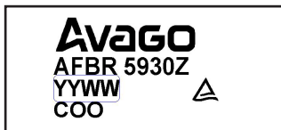
Figure 2b. Component Labeling information
