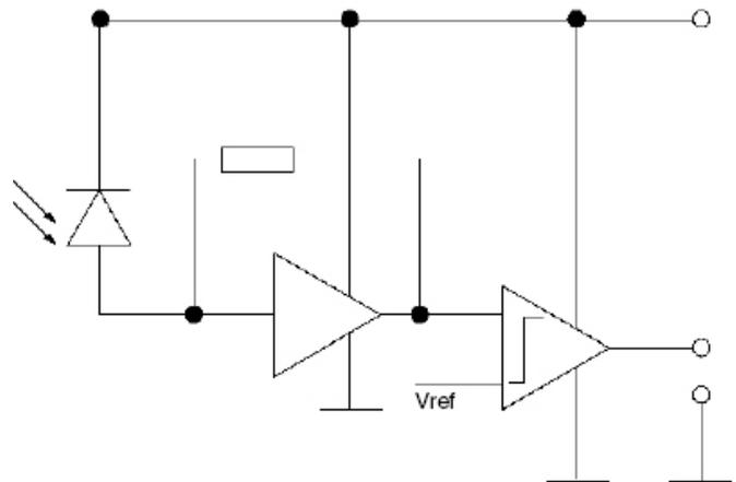
Figure 5. DC Coupled Optical Receiver (SFH551/1)
