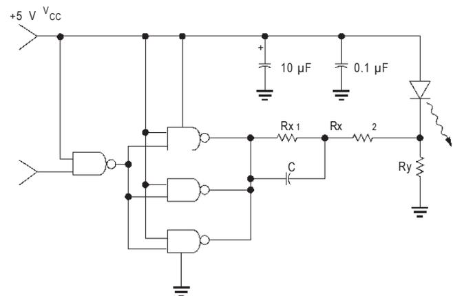
Figure 2. LED Driver with NAND Gates
