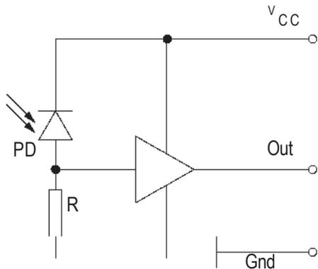
Figure 4. Basic Circuit for Optical Receiver
