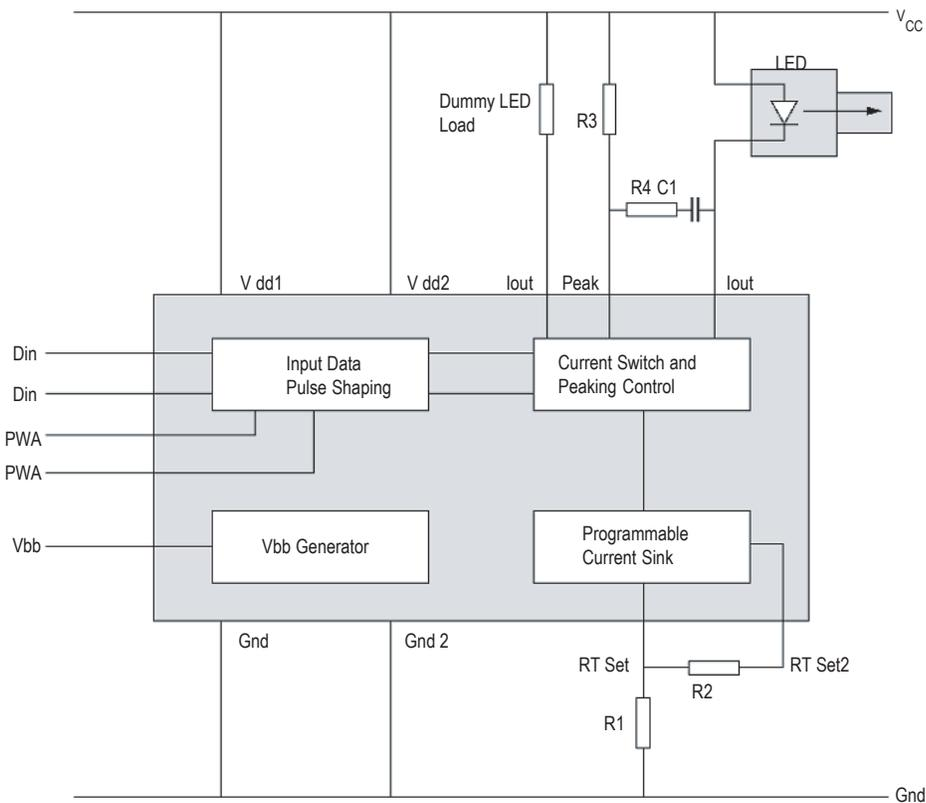
Figure 3. LED Driver from Microcosm
