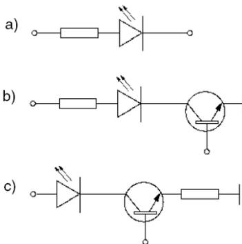
Figure 1. Basic Types of LED Driver Circuits
