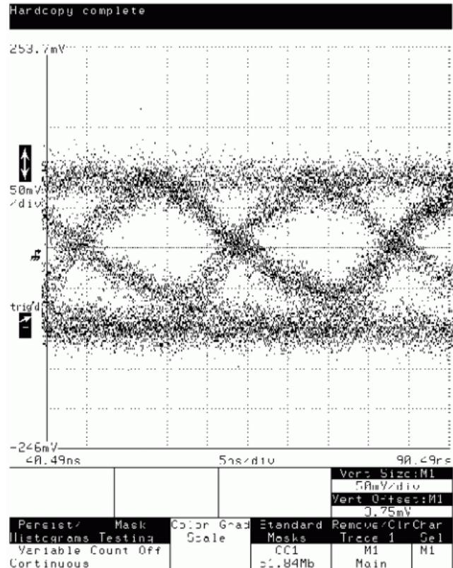
**Figure 8. Eye Diagram at Preamp Output Working with Minimum Optical Power**
