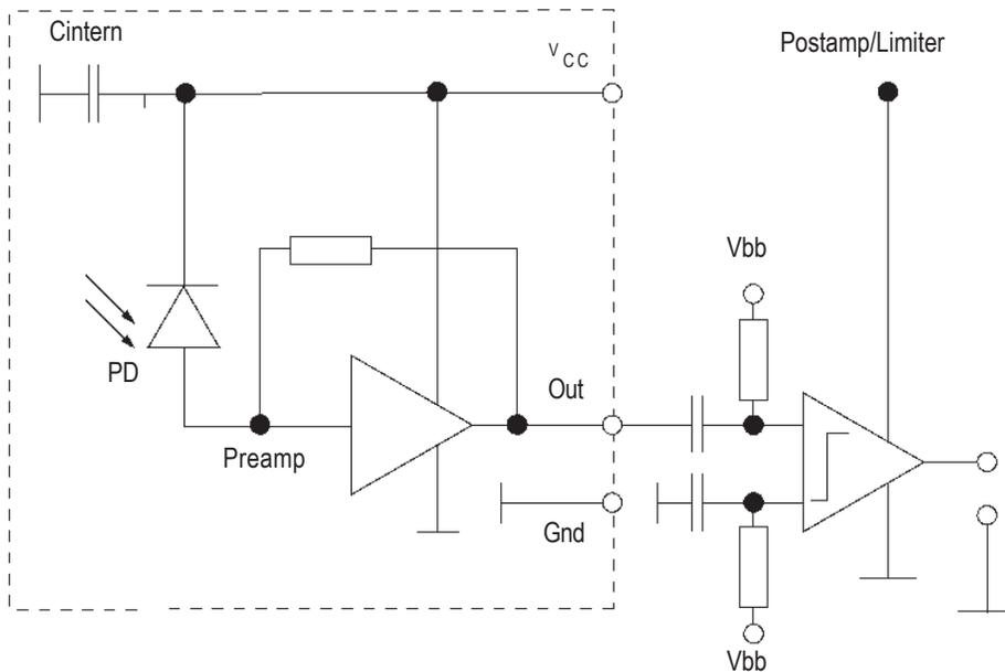
Figure 6. Basic Circuit for AC Coupled Optical Receiver
