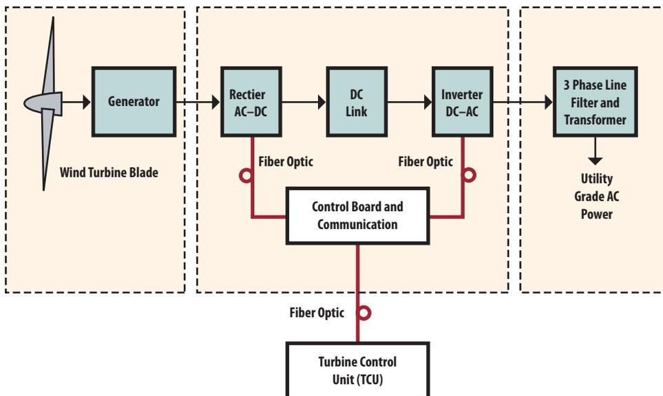
Figure 1. Wind Turbine Power Generation Block Diagram
