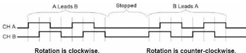
Figure 1. Leading channel at different rotational directions.
