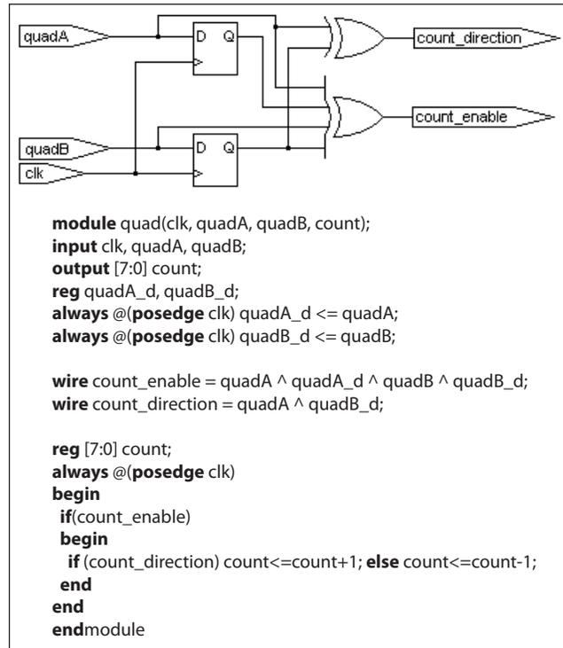
Figure 4. Example of a simplified quadrature decoder using Verilog coding
