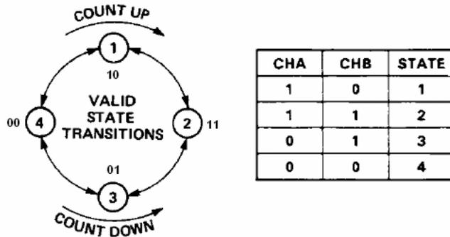
Figure 3. Quadrature signals in 2x and 4x decoding modes
