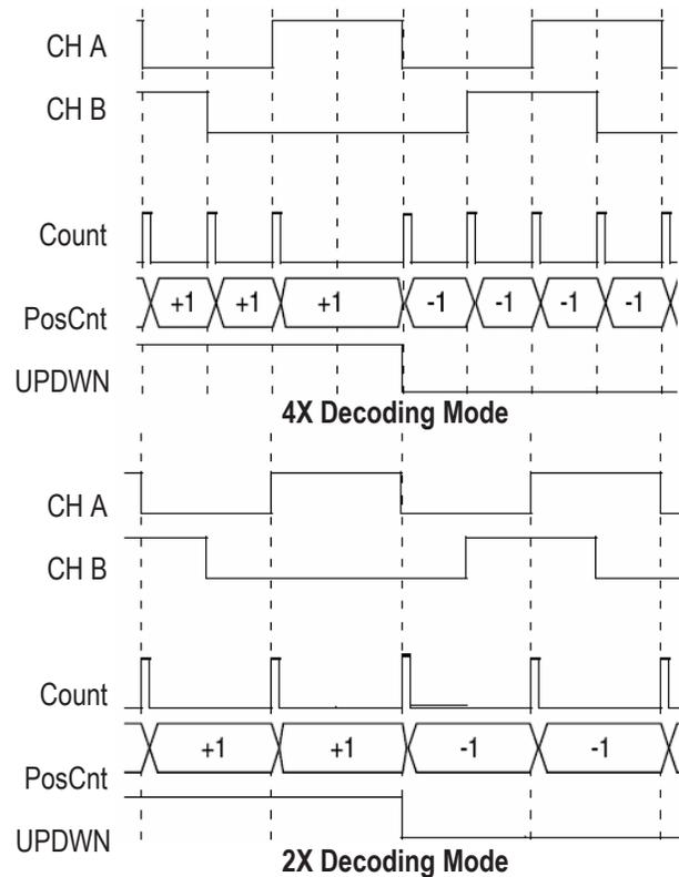
**Figure 2. Quadrature signals in 2x and 4x decoding modes**
