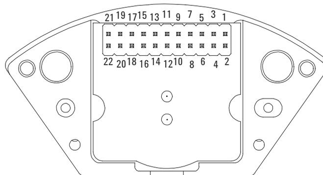
Figure 2. Pinout Configuration
