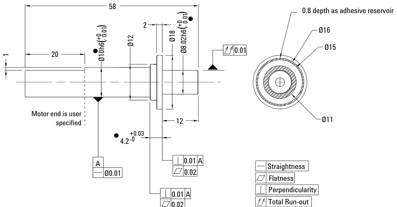
**Figure 5. Design reference for code disk hub-shaft**
