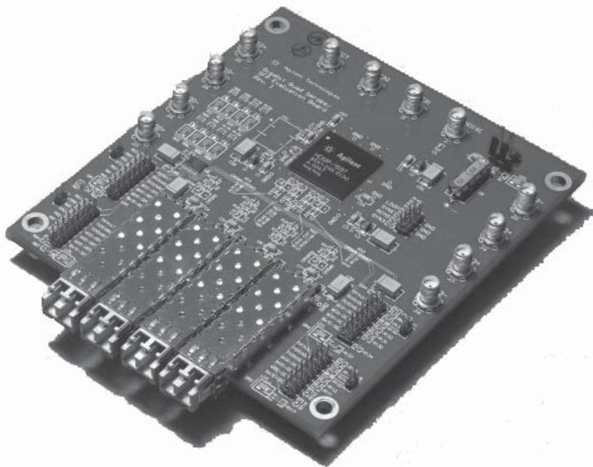
Figure 1. 1.25 GbD reference design PCB including HFBR-5701L/5710L/5720L/5730L (SFP) and HDMP-1687 (Quad SerDes)
