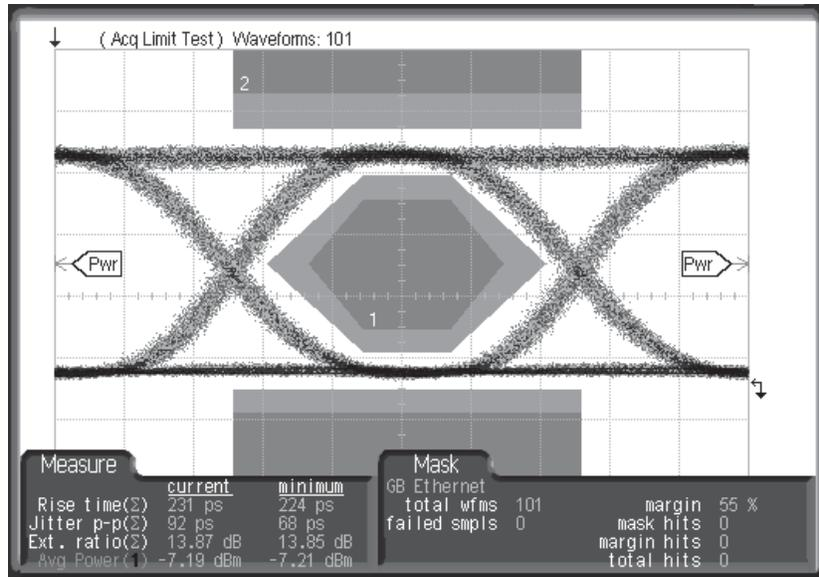
Figure 6. TP02 eye diagram with PRBS 2<sup>7</sup>-1 pattern at 1.25 GBd
