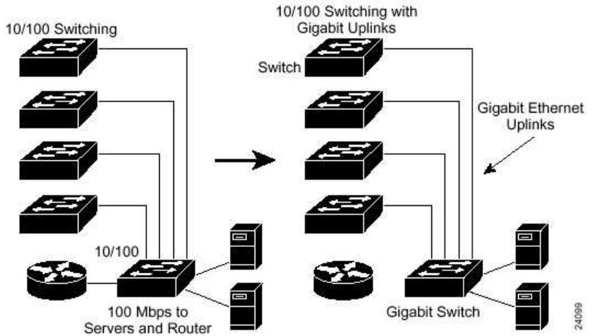
Figure 2. Representative GigaBit Ethernet (GBE) application
