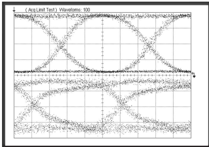
Figure 7. TP02 optical eye diagram and SerDes SO+ electrical eye diagram
