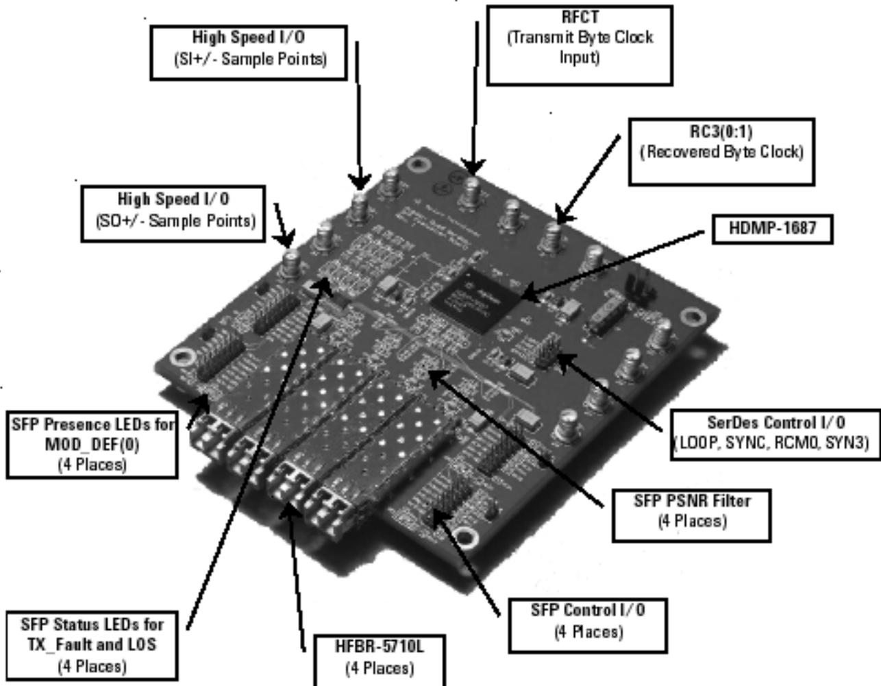
Figure 3. Basic topology of 1.25 Gb/s reference design
