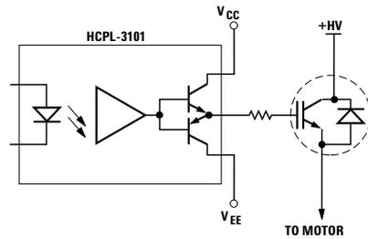
Figure 2b. Isolated Drive Circuit with an HCPL-3100/1 Integrated Gate Drive Optocoupler.
