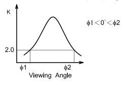
Contrast ratio K vs viewing angle ♦
