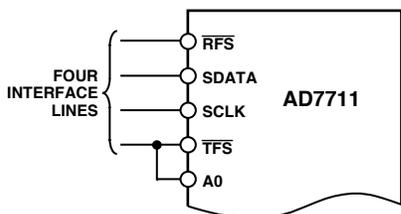
Figure 14. Simplified Interface with  $\overline{\text{TFS}}$  Connected to A0
