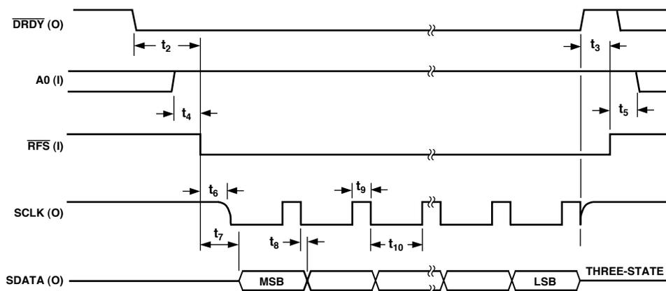
Figure 10. Self-Clocking Mode, Output Data Read Operation
