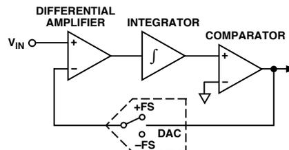
Figure 5. Basic Charge-Balancing ADC
