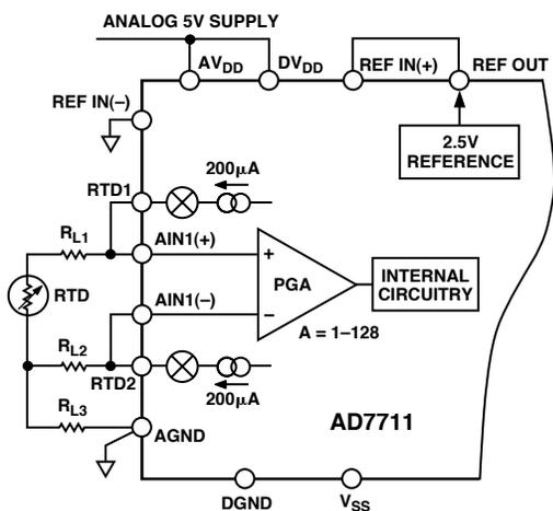
Figure 20. 3-Wire RTD Application with the AD7711
