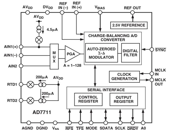
The AD7711 is ideal for use in smart, microcontroller based systems. Gain settings, signal polarity, input channel selection, and RTD current control can be configured in software using the bidirectional serial port. The AD7711 contains self-calibration, system calibration, and background calibration options, and also allows the user to read and write the on-chip calibration registers.
