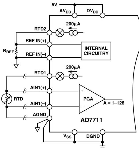
Figure 19. 4-Wire RTD Application with the AD7711
