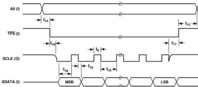
Figure 11. Self-Clocking Mode, Control/Calibration Register Write Operation
