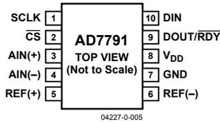
Figure 5. Pin Configuration
