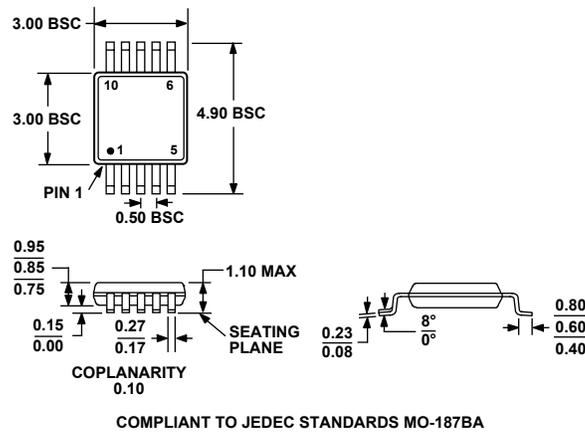
Figure 16. 10-Lead Mini Small Outline Package [MSOP] (RM-10)
