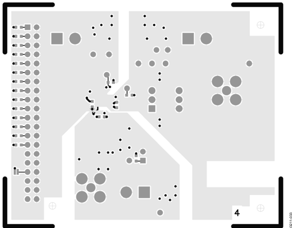
Figure 36. Evaluation Board Layout—Secondary Side
