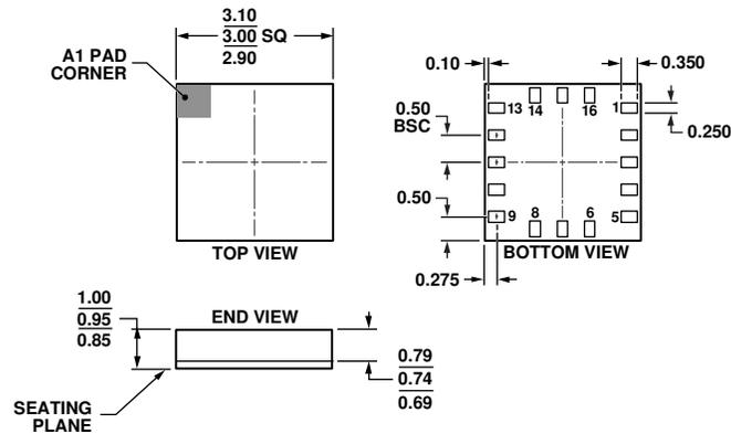
Figure 48. 16-Terminal Land Grid Array [LGA]
