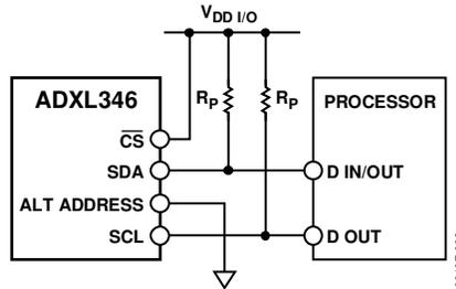
Figure 32. I<sup>2</sup>C Connection Diagram (Address 0x53)
