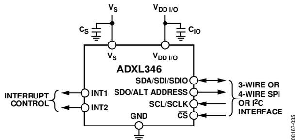
Figure 36. Application Diagram
