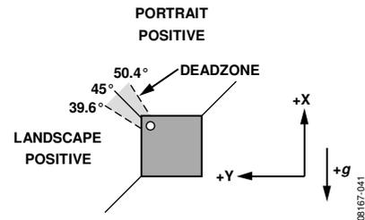
Figure 43. Orientation Showing a 10.8° Dead Zone Region
