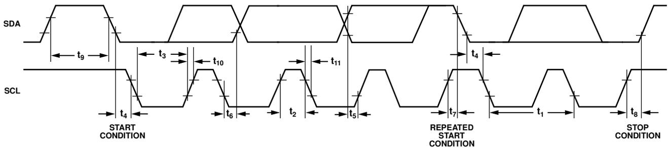
Figure 34. I<sup>2</sup>C Timing Diagram
