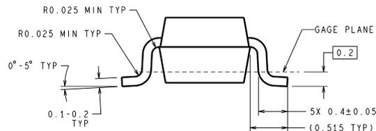
DIMENSIONS ARE IN MILLIMETERS
