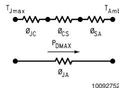
Once the maximum package power dissipation has been calculated using *Equation (1)*, the maximum thermal resistance,  $\theta_{SA}$ , (heat sink to ambient) in °C/W for a heat sink can be calculated. This calculation is made using *Equation (3)* which is derived by solving for  $\theta_{SA}$  in *Equation (2)*.
