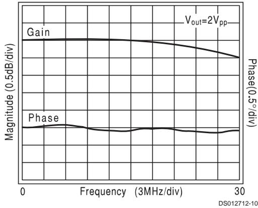
**Differential Gain and Phase at 3.58MHz**
