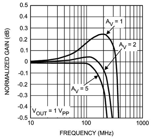
**Typical Performance Characteristics**  $A_V = +2$ ,  $V_{CC} = \pm 5V$ ,  $R_L = 100\Omega$ ,  $R_F = 549\Omega$ ; unless otherwise specified). (Continued)
