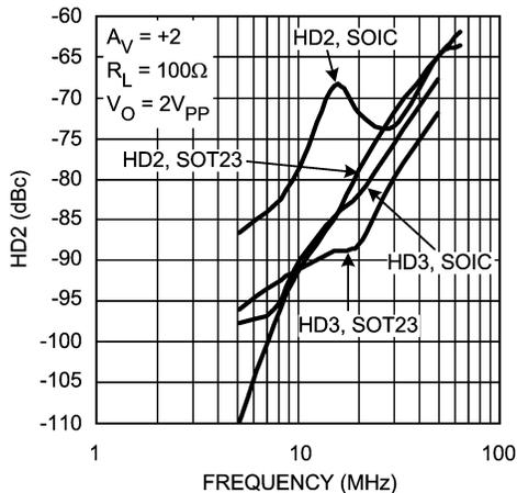
**FIGURE 4. SOIC and SOT23-5 Packages Distortion Terms Compared**
