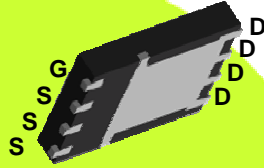
QFN 5mm x 6mm Plastic Package
