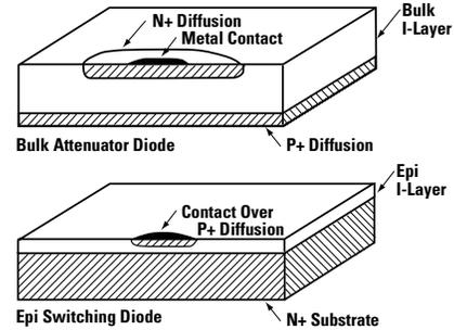
Figure 9. PIN Diode Construction.
