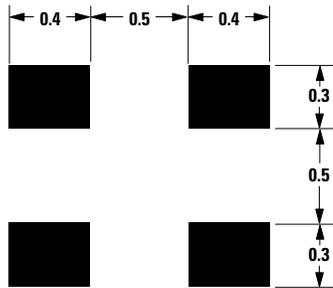
Figure 21. PCB Pad Layout, MiniPak (dimensions in mm).
