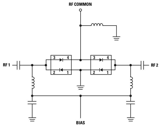
**Figure 7. High Isolation SPDT Switch Using Dual Bias.**
