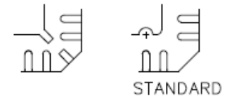
DETAIL A PIN #1 ID AND TIE BAR MARK OPTIONS
