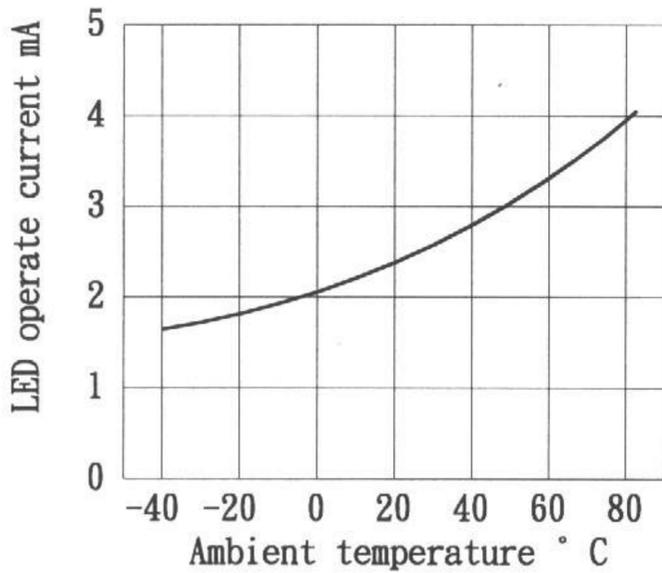
LED turn off current vs. ambient temperature
