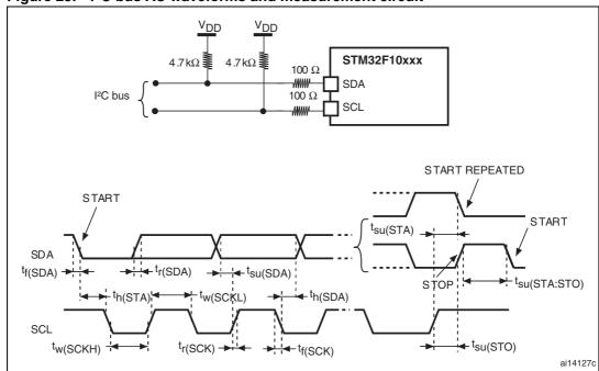
Figure 23. I<sup>2</sup>C bus AC waveforms and measurement circuit<sup>(1)</sup>
