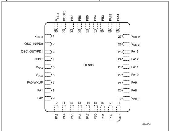
Figure 6. STM32F101xx access line VFQPFN36 pinout
