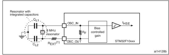
Figure 19. Typical application with an 8 MHz crystal
