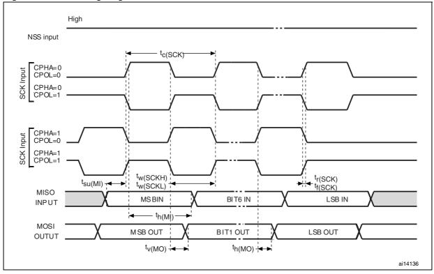
Figure 26. SPI timing diagram - master mode<sup>(1)</sup>
