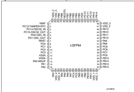
Figure 4. STM32F101xx Medium-density access line LQFP64 pinout
