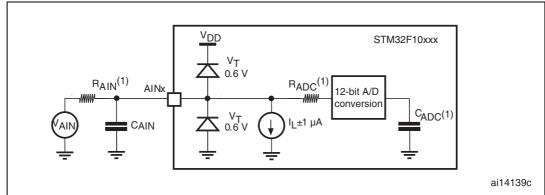
Figure 28. Typical connection diagram using the ADC
