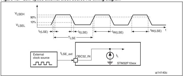
Figure 18. Low-speed external clock source AC timing diagram
