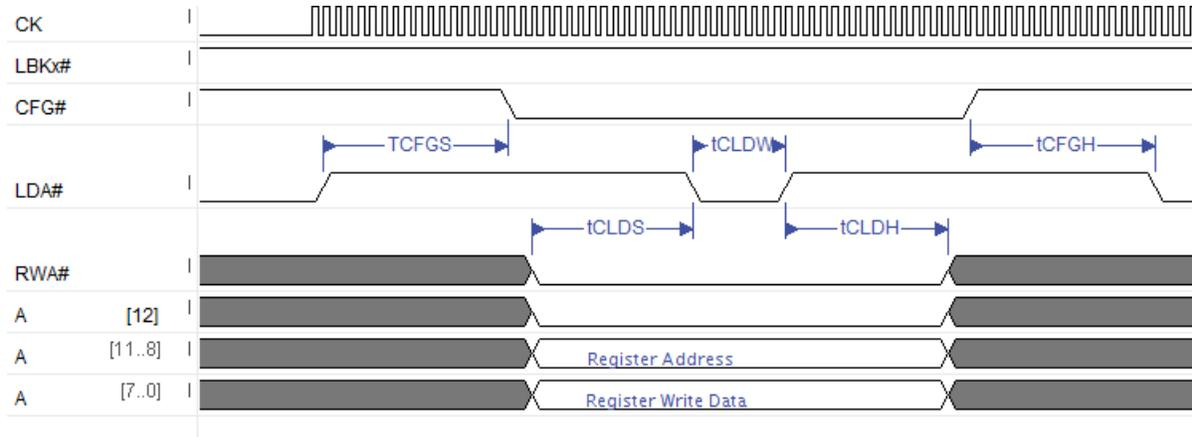
Figure 13. Configuration Read Timing Waveform
