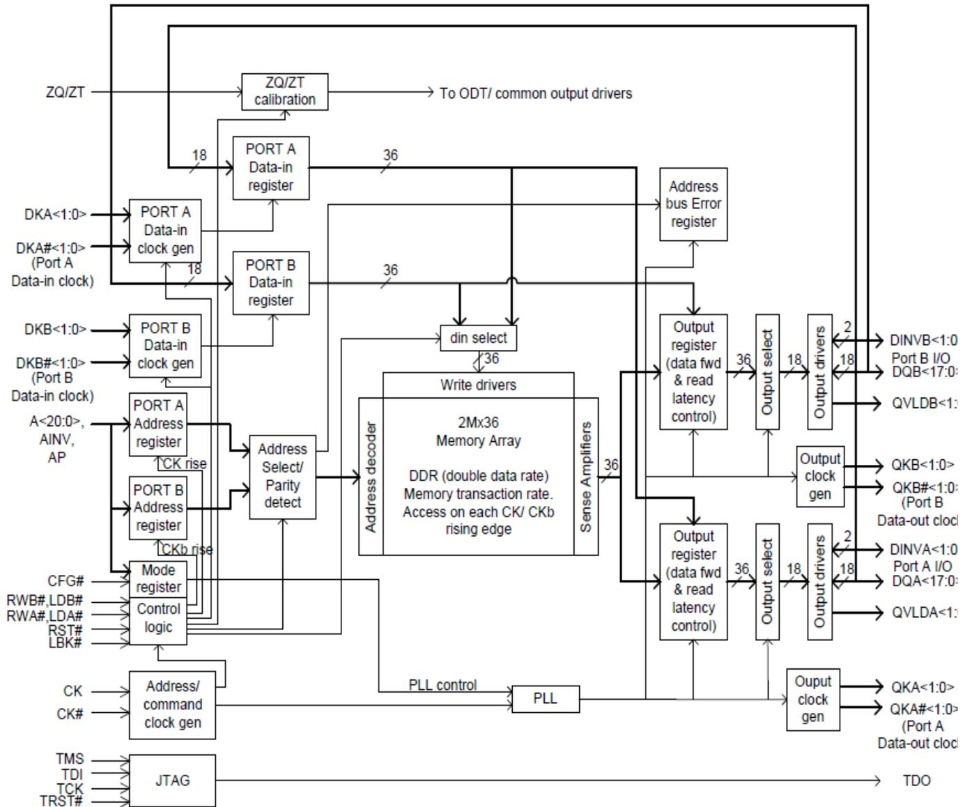
Logic Block Diagram – CY7C4042KV13
