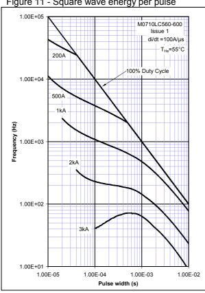
Figure 12 - Square wave energy per pulse
