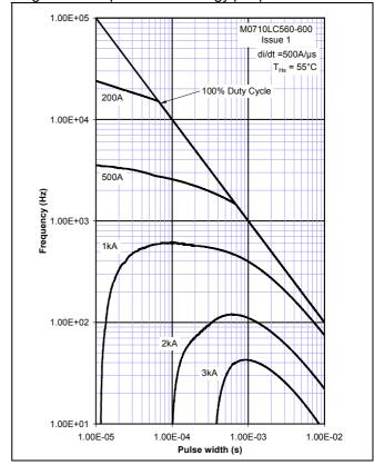
Figure 13 - Square wave frequency vs. pulse width
