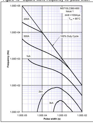
Figure 14 - Square wave frequency vs. pulse width
