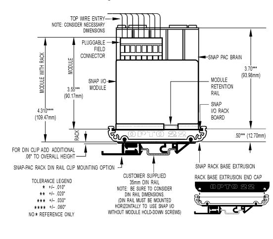
**SNAP Digital Module Mounted on SNAP Rack**
