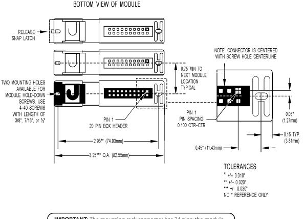
**IMPORTANT:** The mounting rack connector has 24 pins; the module connector has 20 pins. The extra pins on the mounting rack connector prevent misalignment of the module during installation.
