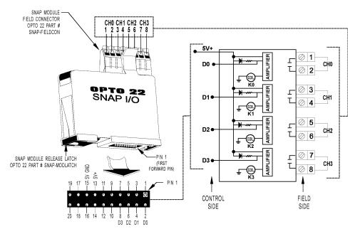
SNAP DIGITAL MODULE BASE CONTROL CONNECTOR (BOTTOM VIEW)
