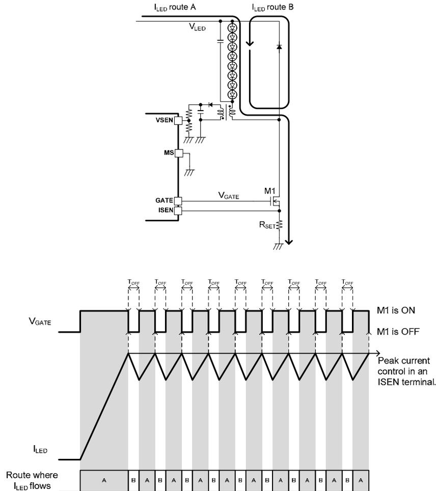
When  $I_{LED}$  route A detected with the ISEN terminal rises to the set peak current value, M1 is turned off. And when  $T_{OFF}$  has passed since M1 turned off, M1 is turned on again. The peak current value can be set up with LD terminal input voltage. (Please refer to page 12 for details.)  $T_{OFF}$  is decided according to the voltage generated on secondary side voltage of a transformer. Secondary side voltage is stabilized in (total  $V_f$  of LED) + ( $V_f$  of diode).
