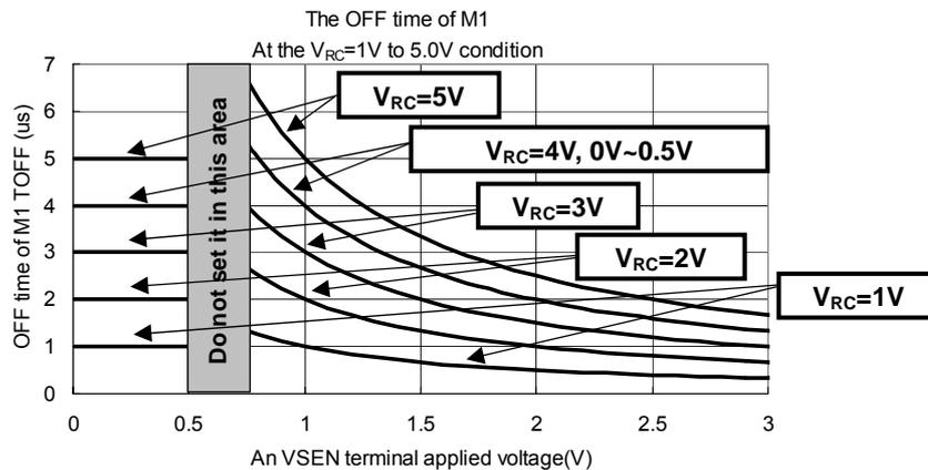
Please use the input voltage to a VSEN terminal in  $0V \sim 0.5V$  or  $0.75V \sim 3.0V$ .
