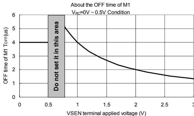
Please use the input voltage to a VSEN terminal in 0V~0.5V or 0.75V~3.0V.
