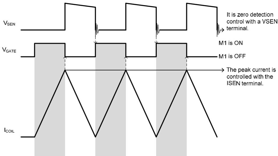
When AC voltage waveform is input to a LD terminal,  $I_{COIL}$  waveform is made a waveform similar to AC voltage waveform. The power factor can be improved by this.
