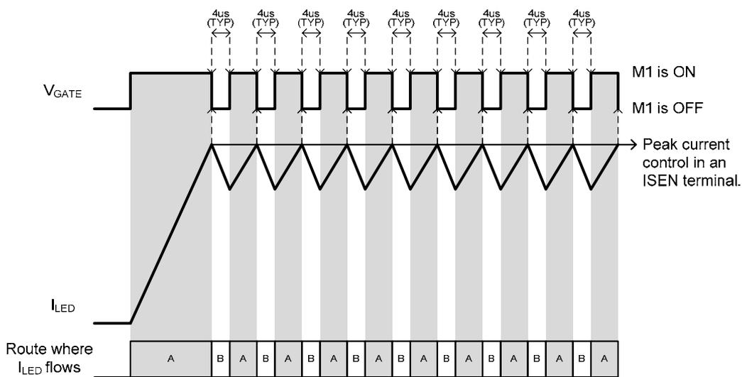
When  $I_{LED}$  route A detected with the ISEN terminal rises to the set peak current value, M1 is turned off. And when 4μs (TYP) has passed since M1 turned off, M1 is turned on again. The peak current value can be set up with LD terminal input voltage. (Please refer to page 12 for details.)
