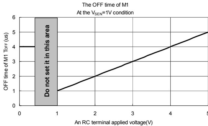
Please use the input voltage to a RC terminal in  $0V \sim 0.5V$  or  $1.0V \sim V_{REG}$ .
