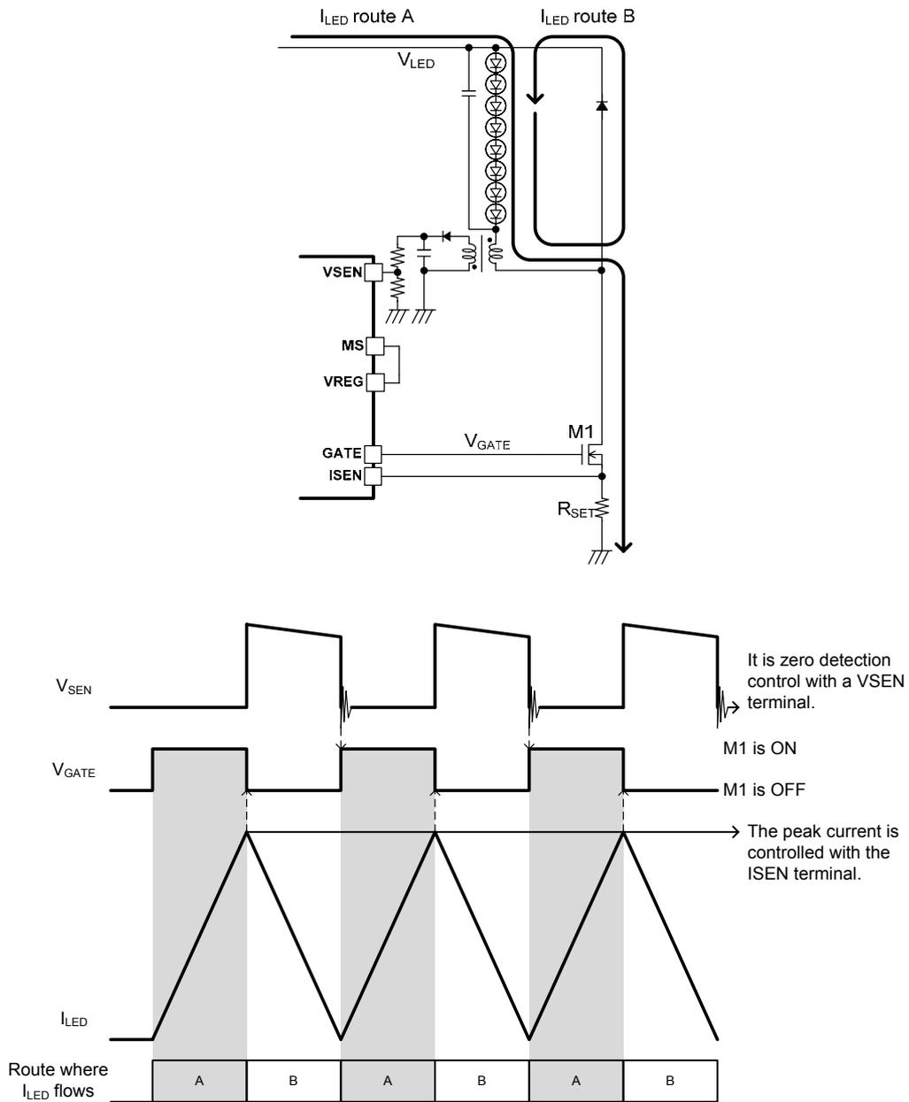
When  $I_{LED}$  route A detected with the ISEN terminal rises to the set peak current value, M1 is turned off.  $I_{LED}$  route B = 0mA is detected by zero detection on the secondary side of the transformer, and M1 is turned on again. The peak current value can be set up with LD terminal input voltage. (Please refer to page 12 for details.)
