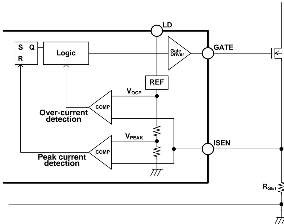
About a setup of  $V_{OCP}$  and  $V_{PEAK}$
