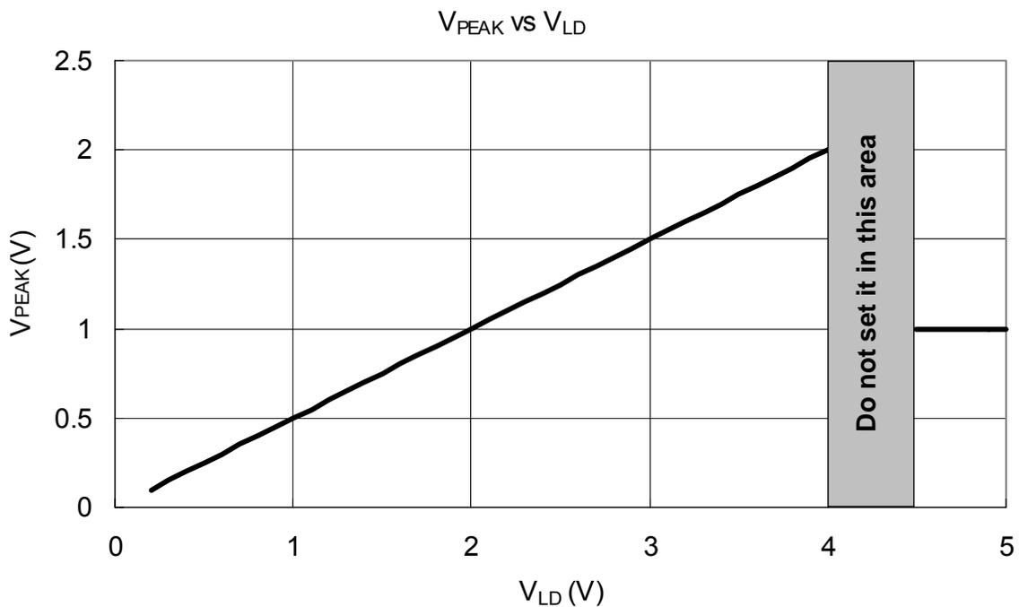
Please use the input voltage to a LD terminal in 0.2V~4.0V or 4.5V~ $V_{REG}$ .
