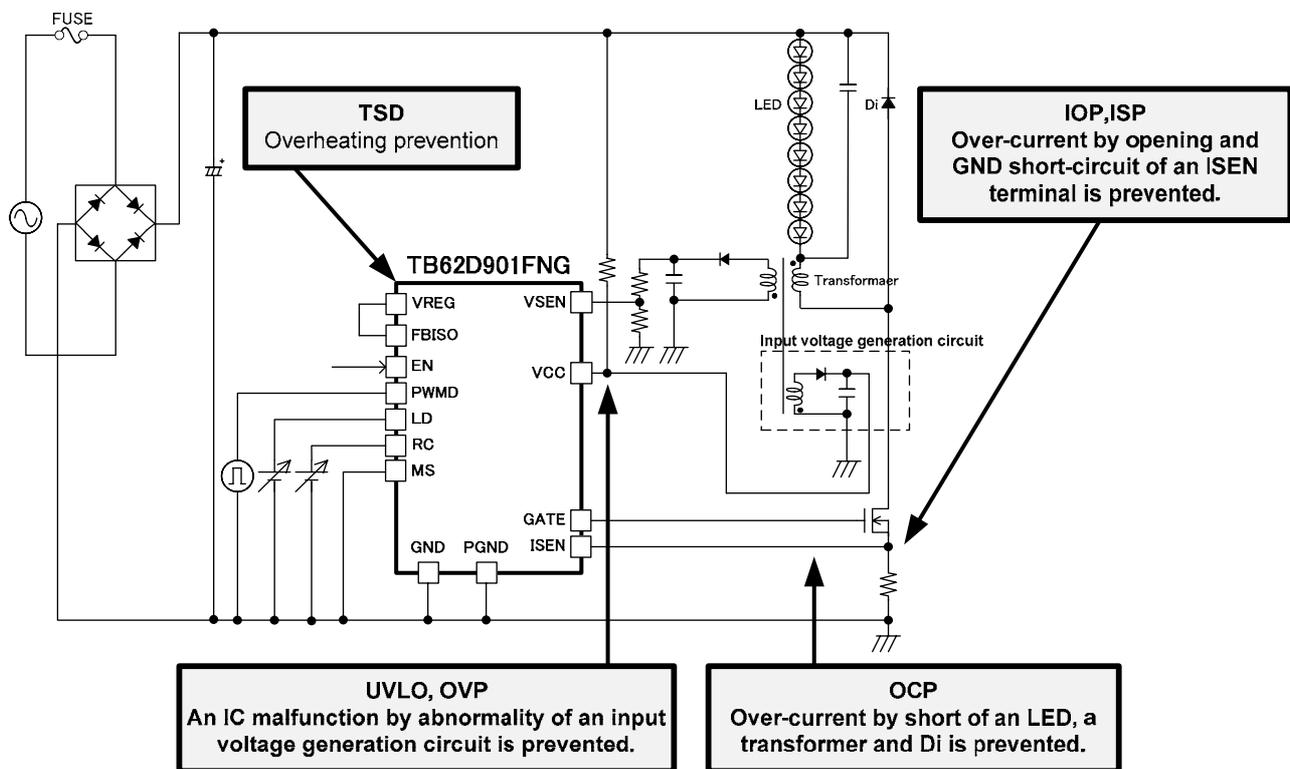
When abnormal voltage occurred by an input voltage generation circuit, the switching control of power MOS is stopped, and the input voltage generation is stopped. The OVP function prevents applying voltage more than absolute maximum ratings to VCC.
