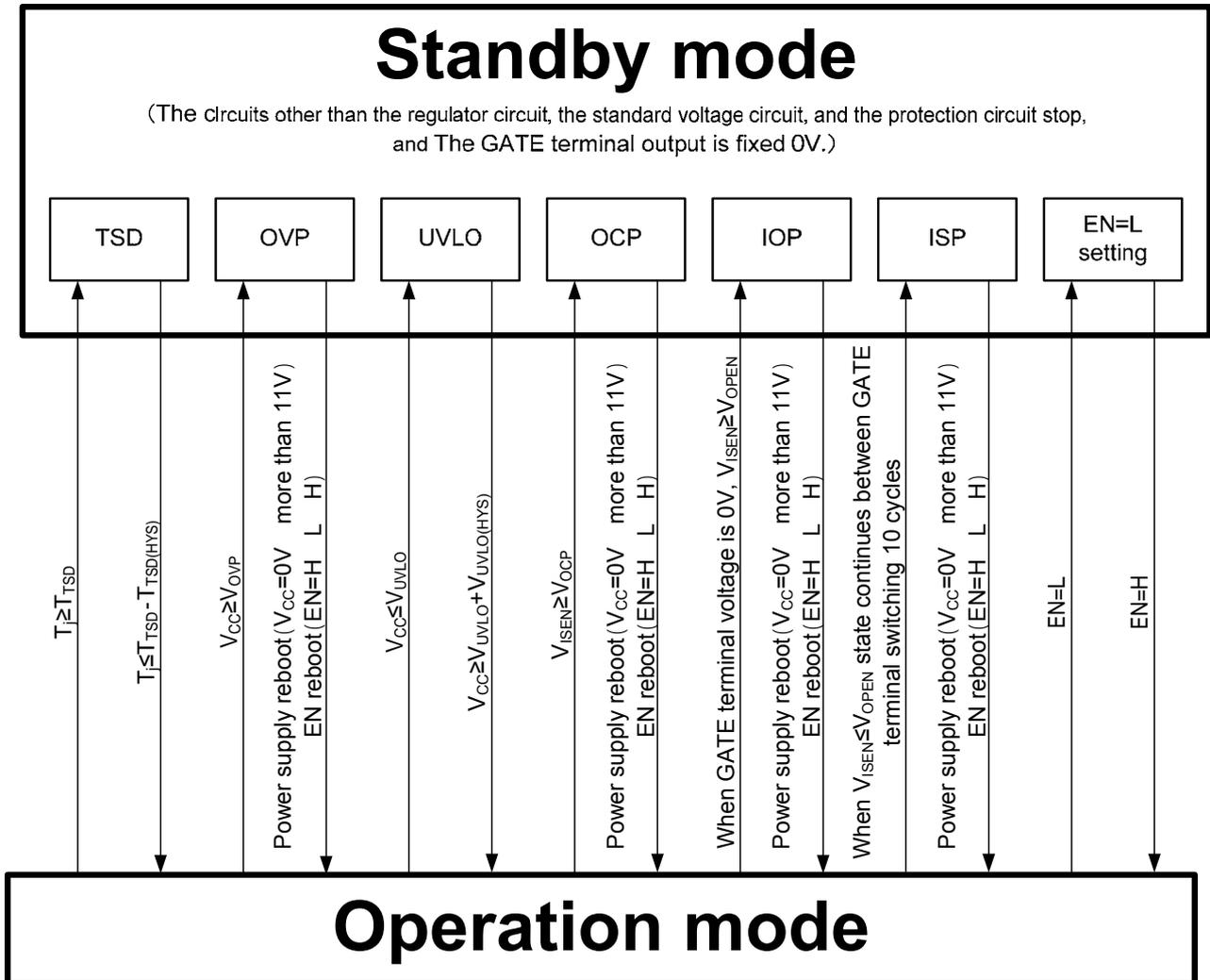
It becomes a standby mode when entering the state that corresponds to either the detection conditions of each protection function or EN=L condition. When corresponding to two or more conditions, unless the condition resolvable of each item is filled, it does not change to normal operation mode.
