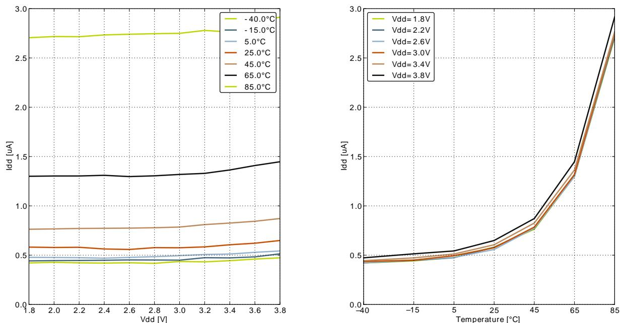
**Figure 3.13. EM4 current consumption.**
