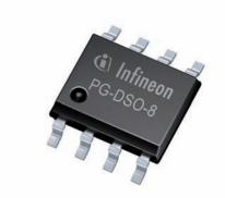
THE TLE5011 is a 360° angle sensor, which detects the orientation of a magnetic field. This is achieved by measuring sine and cosine angle components with monolithic integrated Giant Magneto Resistance elements (iGMR). The data communication is accomplished via a bi-directional Synchronous Serial Communication (SSC) Interface that is SPI compatible.
