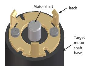
CAUTION: For optimal performance, all the 3 sets of latches should not be subjected to more than 1.5mm outward bending. Excessive outward bending will affect the subsequent, latch to plastic housing grip effectiveness.
