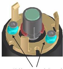
Highly recommended to apply glue to this area to prevent screw loosening, due to the effect of high temperature on plastic.
