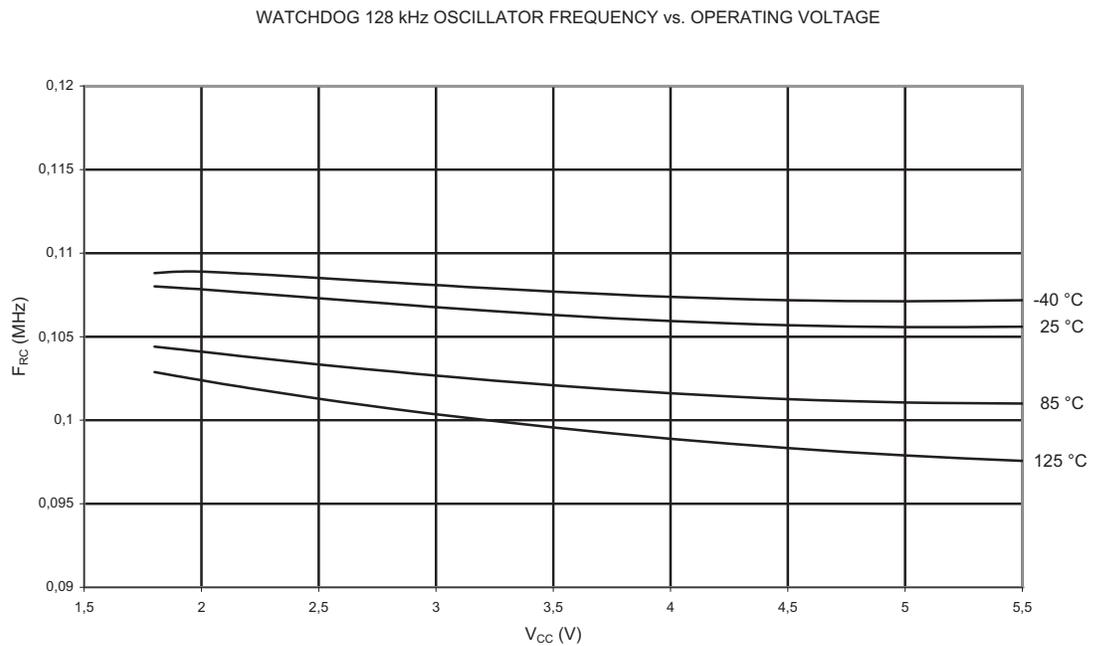
**Figure 2-32.** Calibrated Oscillator Frequency vs.  $V_{CC}$
