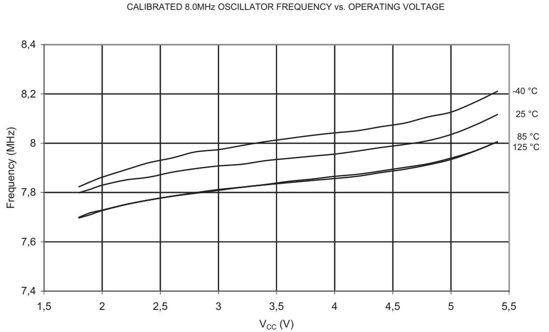
**Figure 2-33.** Calibrated Oscillator Frequency vs. Temperature
