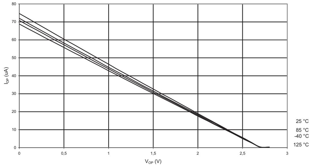
**Figure 2-11.** I/O pin Pull-up Resistor Current vs. Input Voltage ( $V_{CC} = 5V$ )
