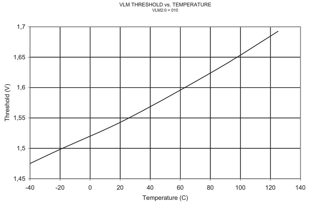
**Figure 2-37.** VLM2 Threshold of  $V_{CC}$  Level Monitor
