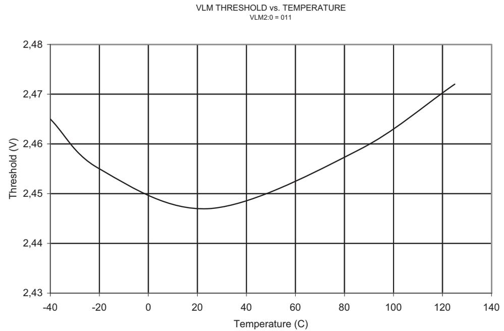
Figure 2-38. VLM3 Threshold of  $V_{CC}$  Level Monitor
