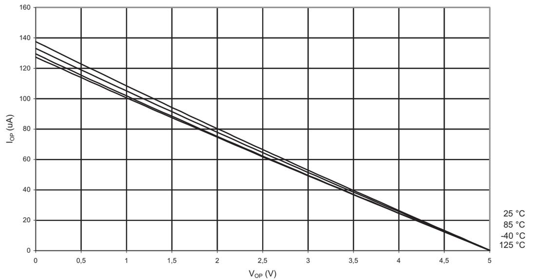
**Figure 2-12.** Reset Pull-up Resistor Current vs. Reset Pin Voltage ( $V_{CC} = 1.8V$ )
