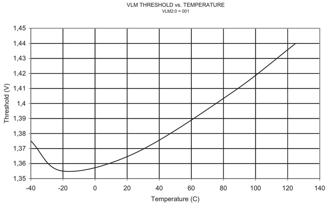
**Figure 2-36.** VLM1H Threshold of  $V_{CC}$  Level Monitor
