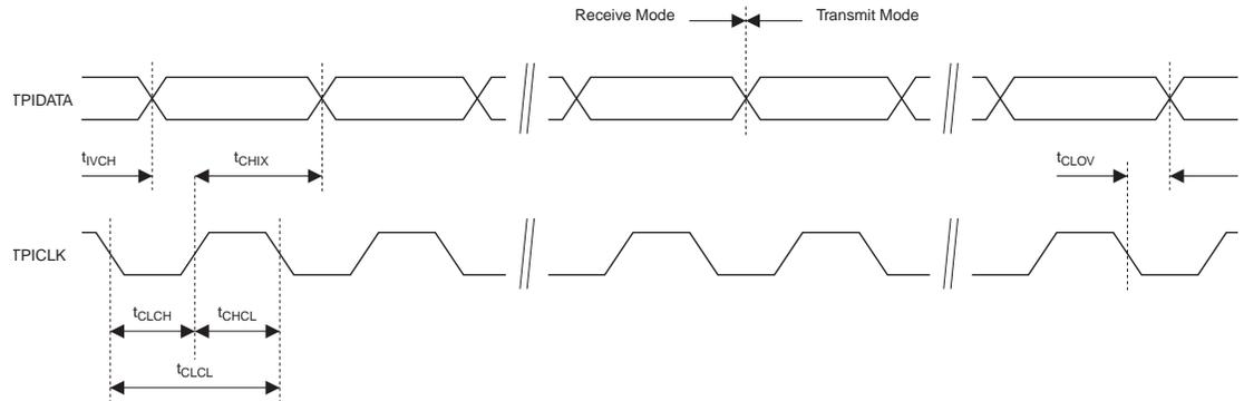
**Table 1-9.** Serial Programming Characteristics,  $T_A = -40^\circ\text{C}$  to  $125^\circ\text{C}$ ,  $V_{CC} = 5\text{V}$  (Unless Otherwise Noted)
