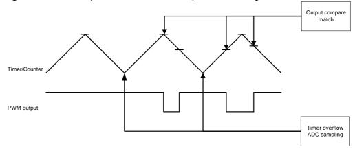
Figure 3-3. PWM output of Timer/Counter in up-down counting mode.
