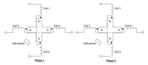
The commutation of two-phase BLDC motors is usually controlled by the use of a Hall sensor to detect the orientation of the rotor. A hall sensor is a magnetic switch, which
