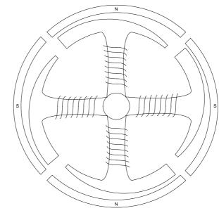
The fundamental two-phase motor of Figure 2-1 does not guarantee the direction of rotation when starting the motor. The direction is determined by the starting position of the rotor and the coil activation order. If the starting position of the rotor is known, the coil activation order that will result in a particular direction of rotation can be determined.
