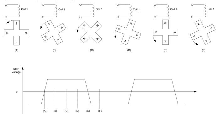
The down side to using the EMF to sense determine the orientation of the rotor is that the EMF amplitude depends on the speed of the motor and there is a practical lower limit to how small voltage levels that can be measured – also considering the noise that will be present in a given system.
