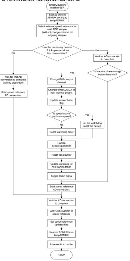
Figure 4-3. Timer/counter0 interrupt service routine.
