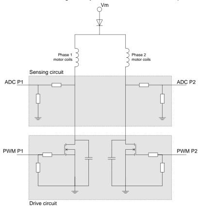
Figure 3-1. Drivers and sensing circuitry for sensorless control of two-phase BLDC
