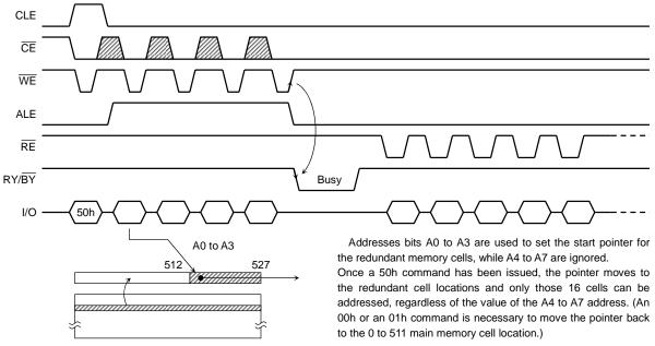
Figure 4. Read mode (3) operation
