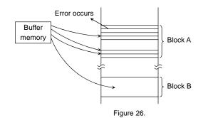
When an error happens in Block A, try to reprogram the data into another Block (Block B) by loading from an external buffer. Then, prevent further system accesses to Block A (by creating a bad block table or by using an another appropriate scheme).
