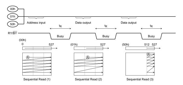
Sequential Read mode (1) and (2) output the contents of addresses 0 to 257 as shown above, while Sequential Read mode (3) outputs the contents of the redundant address locations only.
