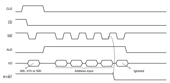
Internal read operation starts when  $\overline{\text{WE}}$  goes High in the fourth cycle.
