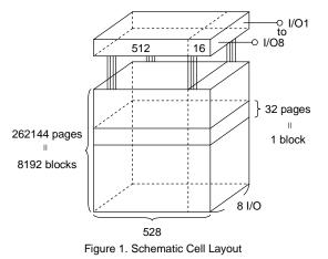
A page consists of 528 bytes in which 512 bytes are used for main memory storage and 16 bytes are for redundancy or for other uses.
