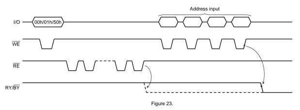
Hence the  $\overline{RE}$  clock input must start after the address input.
