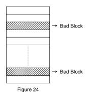
Block, all bytes are not in the FFh state. Please don't perform erase operation to Bad Block. Check if the device has any bad blocks after installation into the system.
