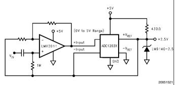
FIGURE 7. AC Coupled ADC Driver
