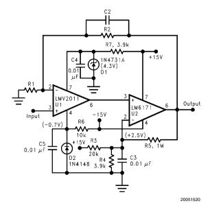
FIGURE 6. Composite Amplifier Configuration
