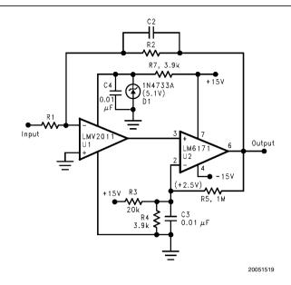
FIGURE 5. Composite Amplifier Configuration
