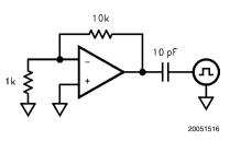
**FIGURE 1. Overload Recovery Test**
