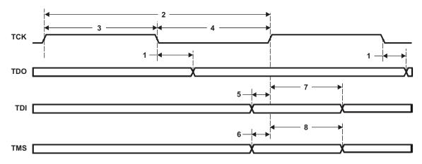
Figure 5-42. JTAG Test-Port Timing
