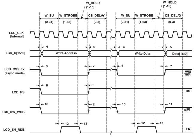
Figure 5-28. Micro-Interface Graphic Display 6800 Write
