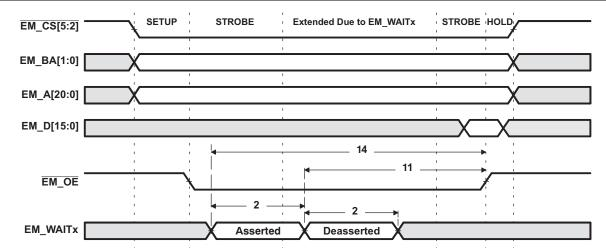
Figure 5-16. EM\_WAITx Read Timing Requirements
