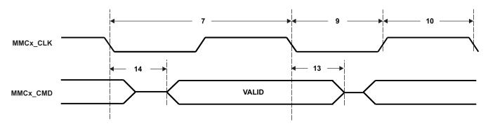
Figure 5-18. MMC/SD Host Command Write Timing
