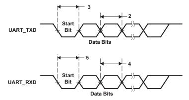
Figure 5-24. UART Transmit/Receive Timing
