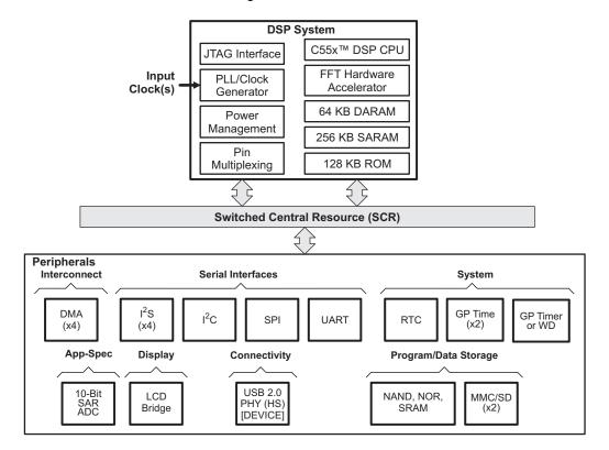
Figure 1-1. TMS320VC5505 Functional Block Diagram
