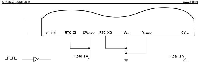
Figure 5-5. LVCMOS-Compatible Clock Input With RTC Oscillator Disabled
