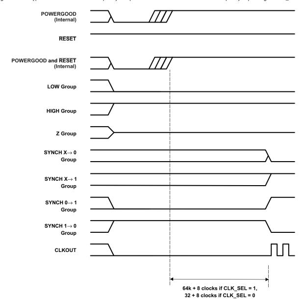
Figure 5-9. Power-On Reset Timing Requirements
