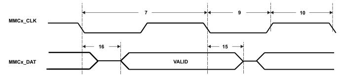
Figure 5-21. MMC/SD Data Write Timing
