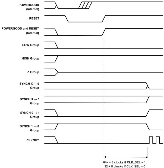
Figure 5-10. Reset Timing Requirements
