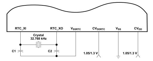
Figure 5-3. 32.768-kHz RTC Oscillator
