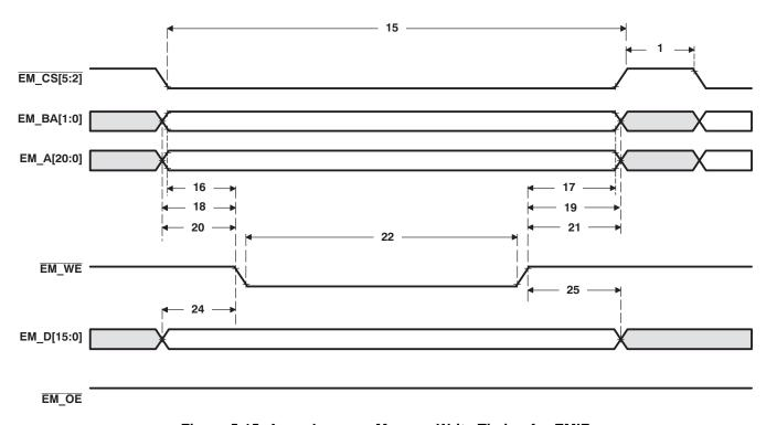
Figure 5-15. Asynchronous Memory Write Timing for EMIF
