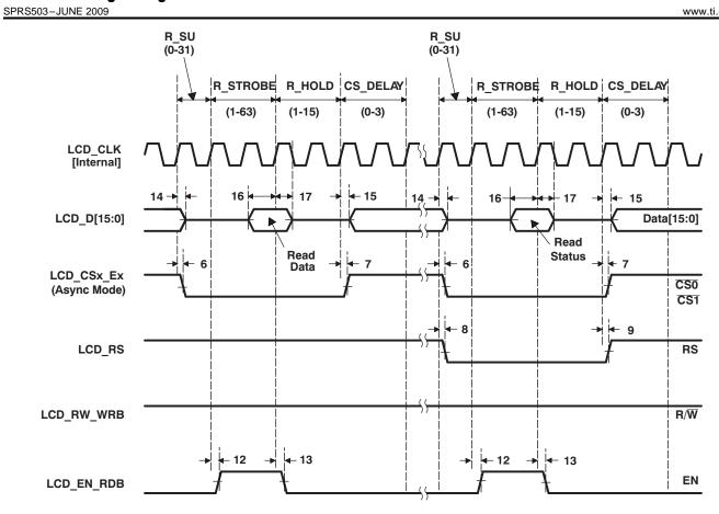
Figure 5-30. Micro-Interface Graphic Display 6800 Status
