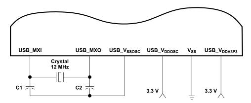
Figure 5-6. 12-MHz USB Oscillator
