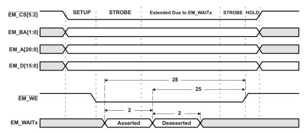
Figure 5-17. EM\_WAITx Write Timing Requirements
