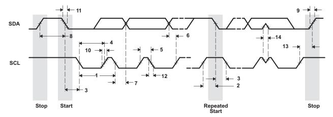
Figure 5-22. I2C Receive Timings
