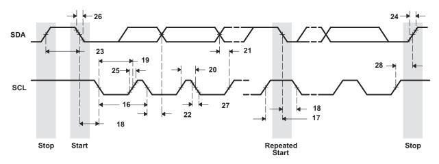
Figure 5-23. I2C Transmit Timings
