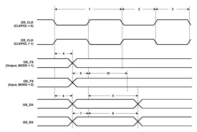
Figure 5-25. I2S Input and Output Timings
