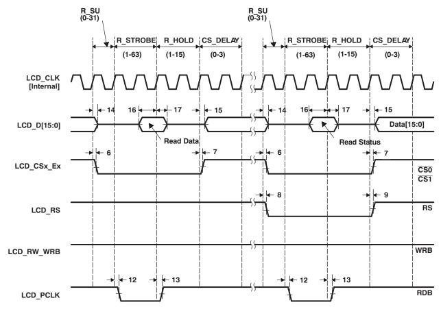
Figure 5-33. Micro-Interface Graphic Display 8080 Status
