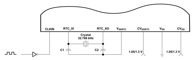
Figure 5-4. LVCMOS-Compatible Clock Input With RTC Oscillator Enabled
