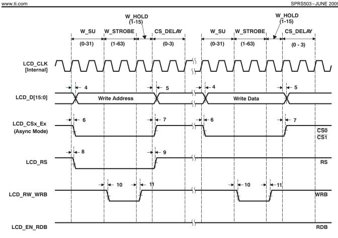
Figure 5-31. Micro-Interface Graphic Display 8080 Write
