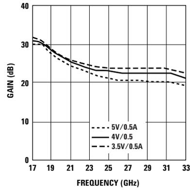
Figure 7. Gain and  $V_{d2}$  voltage,  $V_{d1} = 3.5$  V (constant)
