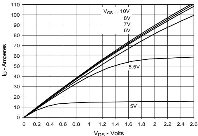
**Fig. 2. Extended Output Characteristics
