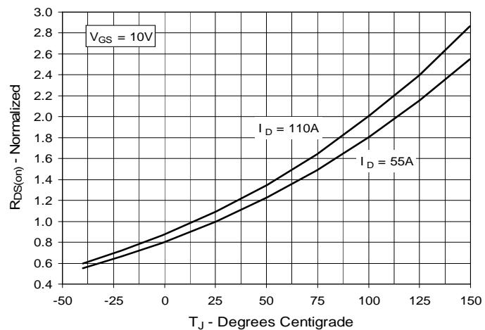
**Fig. 5.  $R_{DS(on)}$  Normalized to  $I_D = 55A$  Value
