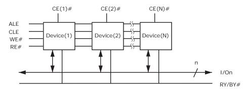
Figure 10.8 Example with Multiple Devices
