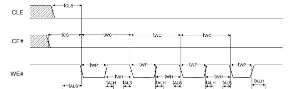
Figure 7.2 Address Latch Cycle Timing Diagram
