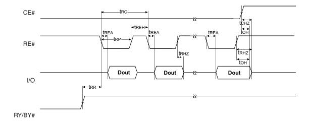
Figure 7.5 Status Read Cycle Timing Diagram
