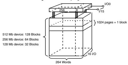
A page consists of 264 Words in which 256 Words are used for main memory storage and 8 Words are reserved for redundancy or other usage.
