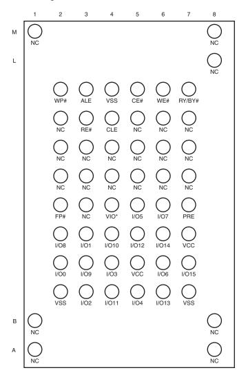
Figure 1.3 55-Ball FBGA Connections - x16
