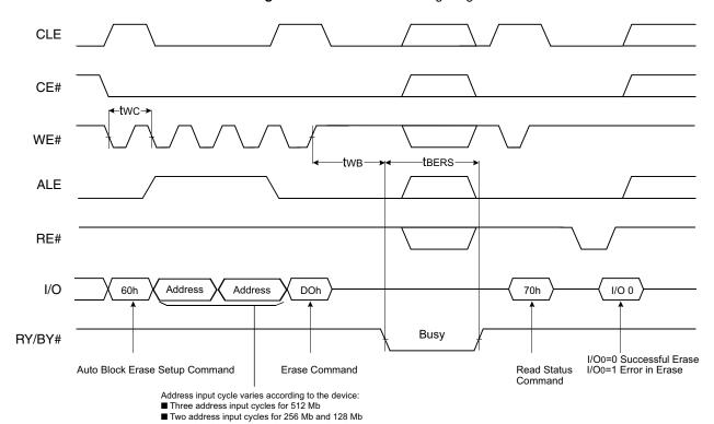
Figure 7.11 Spansion Command Mode Entry Timing Diagram
