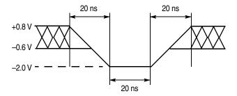
Figure 6.2 Maximum Positive Overshoot Waveform
