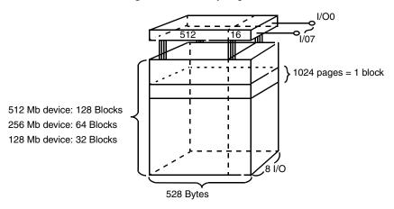
A page consists of 528 Bytes in which 512 Bytes are used for main memory storage and 16 Bytes are reserved for redundancy or other usage.
