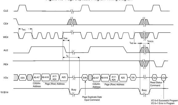
Figure 7.9 Page Duplicate Program Timing Diagram
