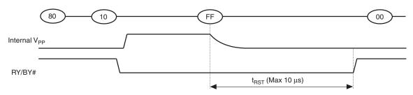
Figure 10.10 Reset (FFh) Command Input During Erasing
